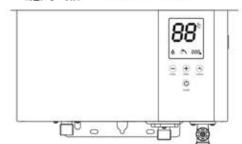
1 從冷水入口拆除濾水器。 Remove the filter at water inlet.
